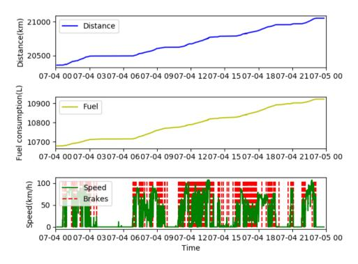
Figure 2. Example of accumulated distance driven (upper), fuel consumption (middle) and speed/breaking activity measured for a vehicle in July 2019.
